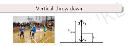
Vertical throw down is a uniformly accelerated rectilinear motion (a = g), in which a body, at a height of h above the ground, is thrown vertically downwards at the initial velocity  $v_0$ .
