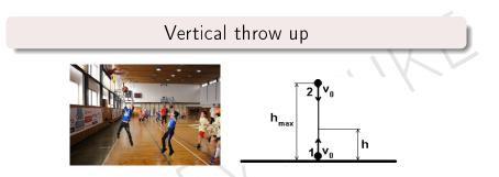
Vertical throw up is a uniformly slowed rectilinear movement (a = g), in which the body, at the surface of the earth, is thrown vertically upwards to a height h at the initial velocity  $v_0$ .
